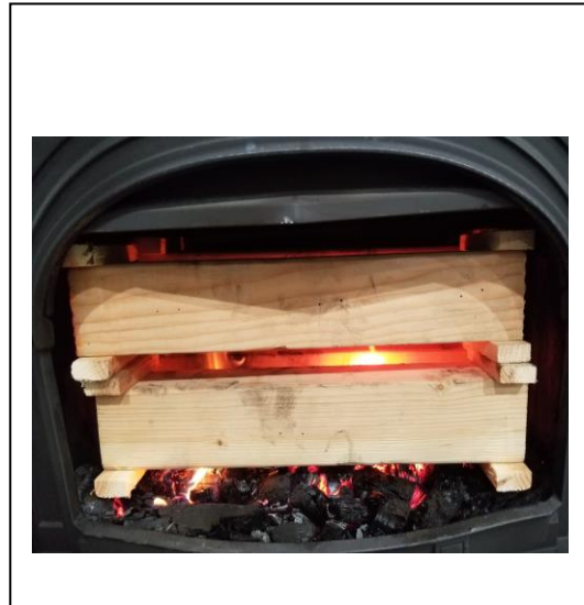
Run 3 – Fuel Loaded in Stove
