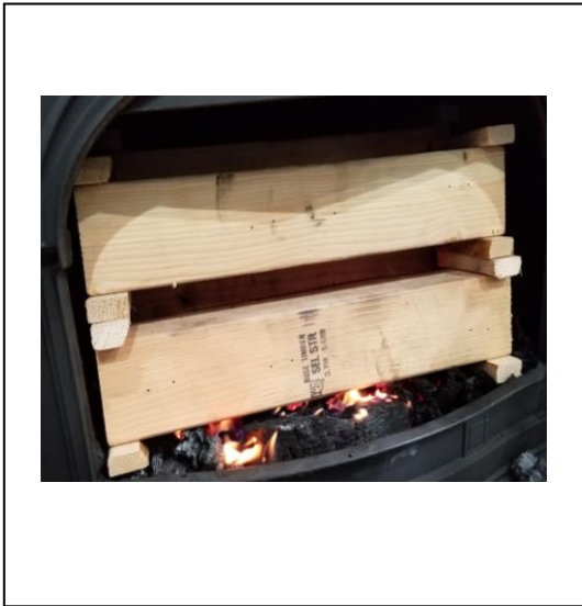
Run 1 – Fuel Loaded in Stove
